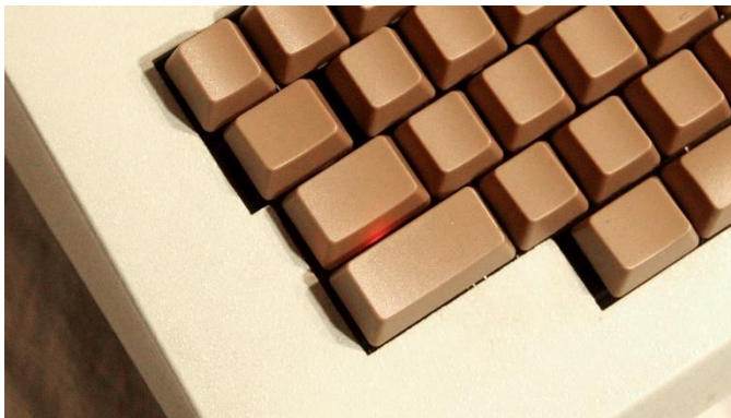
LED Installed under Keycap
