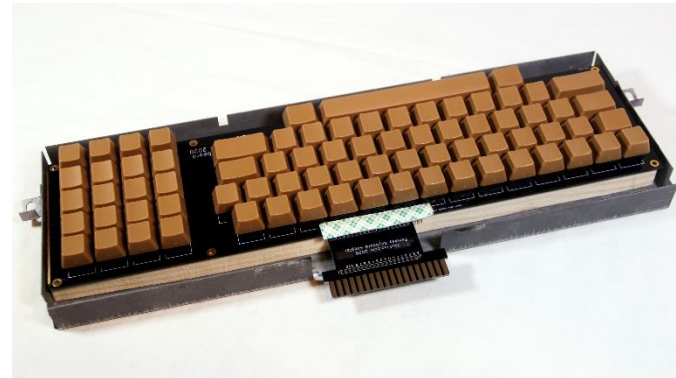
PCB assembly on Top of Housing
