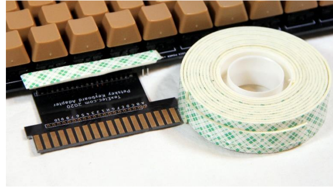
Thick foam Tape used as Insulation
